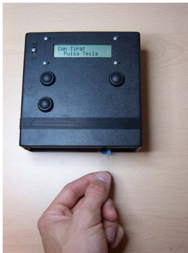
Fig. 7 Photograph of the portable instrument showing how to introduce the disposable sensor
