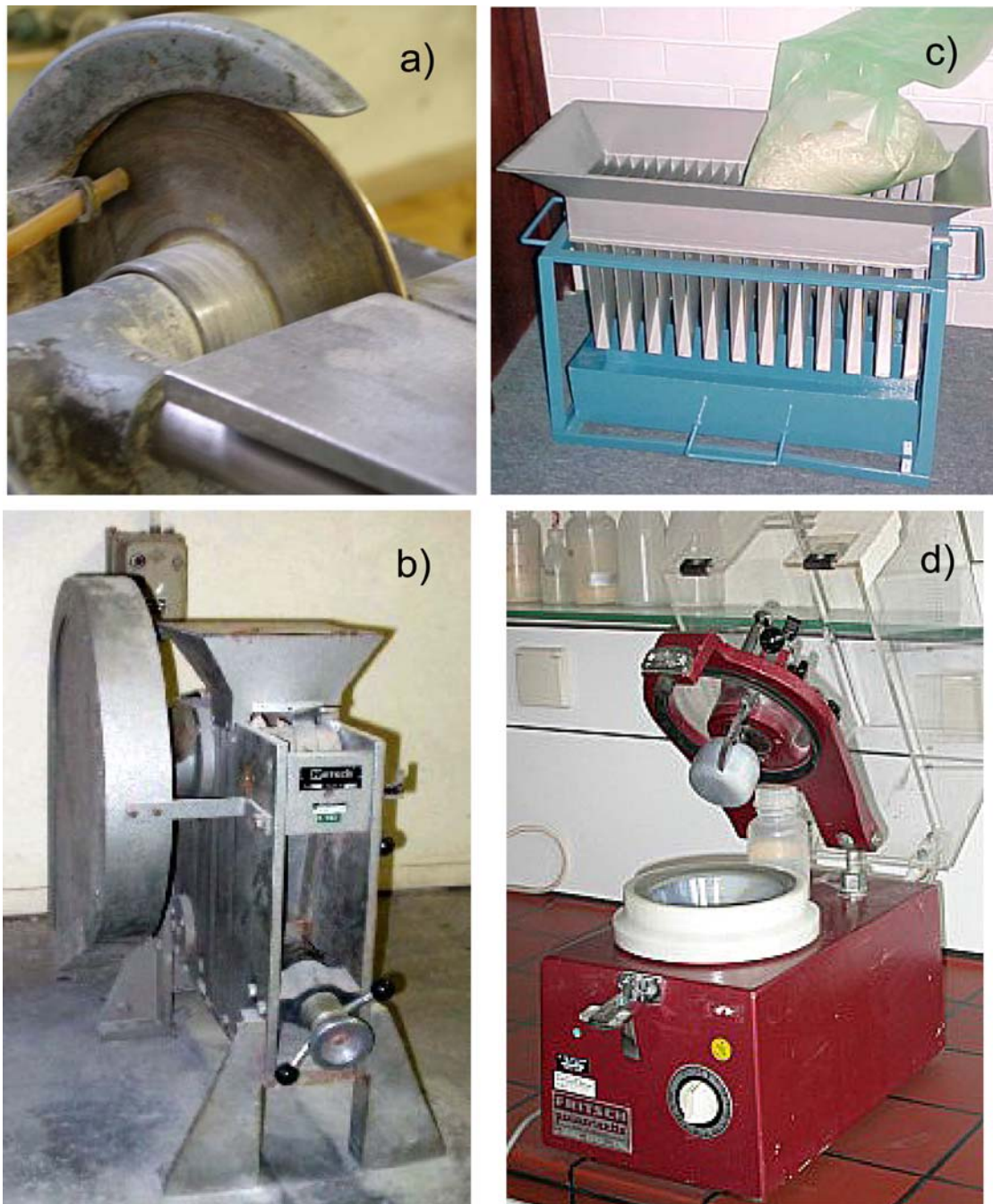
Figure 3.1: Equipment utilized for the preparation of whole rock powders: a) Diamond saw; b) Jaw crusher; c) Riffle-splitter; d) Pulverizer agate mill.
