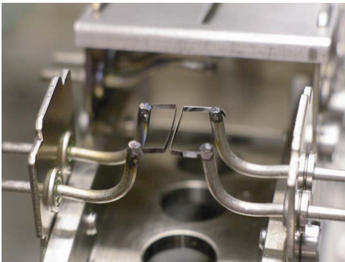
Figure 3.4: Re electric filaments for deposition and loading of samples in TIMS. Photo by V. Bennett, ANU, Canberra (Australia).
