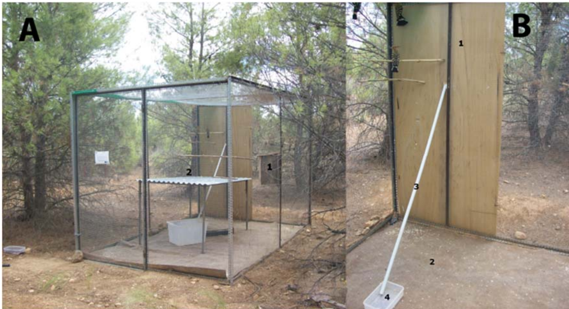
Figure 4. (a) General layout of the cage showing (1) the position of the nestbox and (2) the aluminium roof that protected the food from the weather. (b) Detailed picture of the provisioning equipment showing (1) the wooden panel that hid the researcher, (2) the carpet, (3) the PVC pipe and (4) the plastic feeder.
