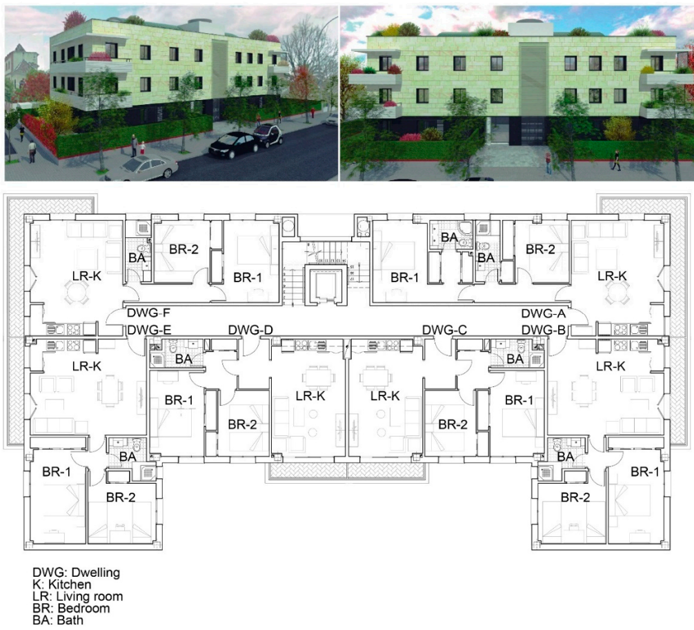
Figure 4. 3D perspective of the case study and the distribution of the typical floor.
