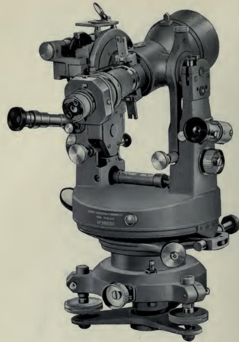
FIG. 11. The Geodetic Tavistock theodolite.
