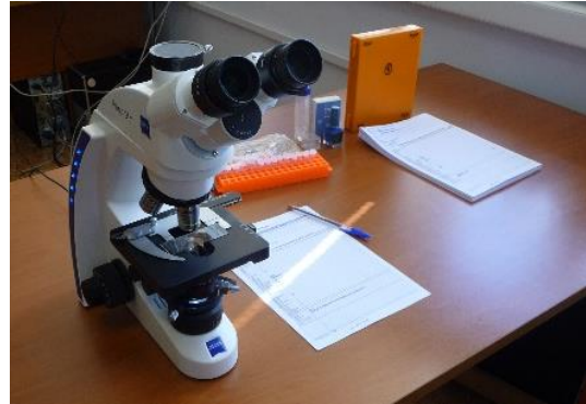
Figure 1.9. Zeiss Transmitted light microscope used for the palynological analysis at the Paleontology and Stratigraphy Department of the University of Granada.
