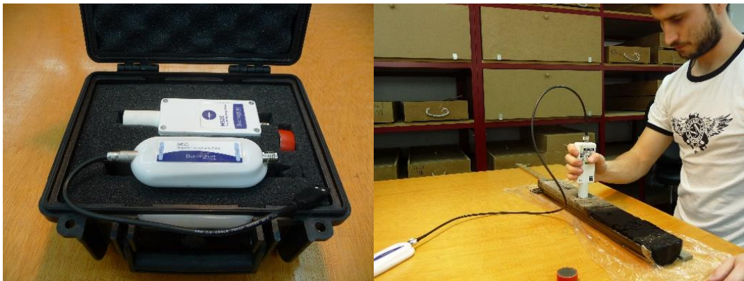
Figure 1.8. Analysis of magnetic susceptibility measured using a Bartington MS3 meter operating with a MS2E manual sensor and connected to a laptop (University of Granada).
