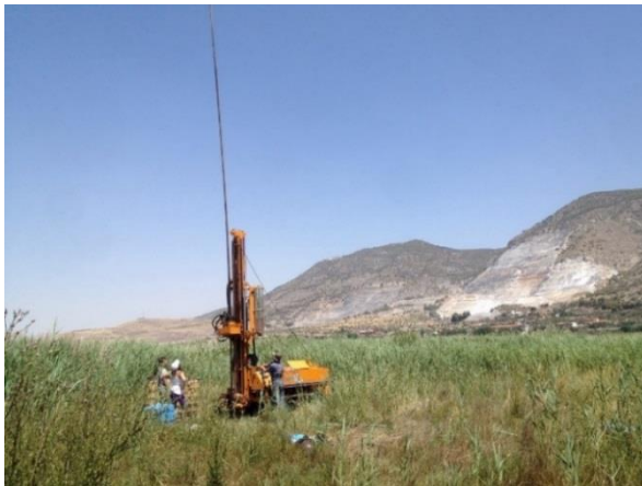
Figure 1.5. Panoramic photography of the coring during July 2015 in the southern edge of the Padul wetland.
