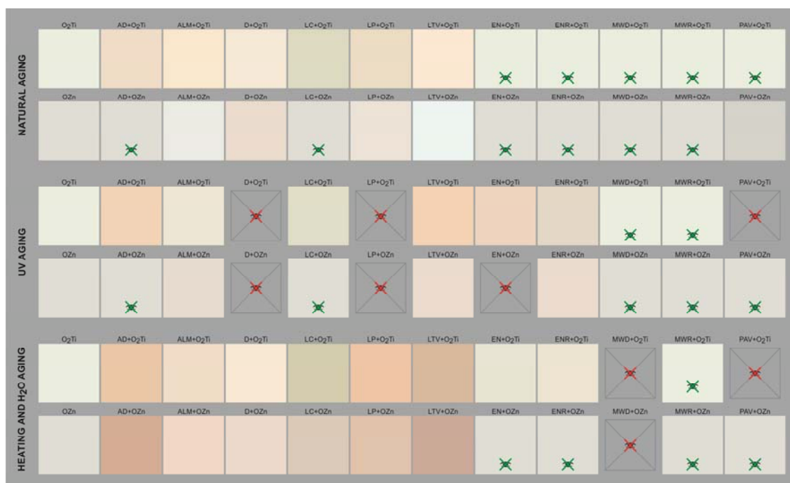
Figure 6. Simulated colour card using the software Spectra Magic de Konica Minolta. The first colour in each series corresponds to the pure pigment. It is followed by colour simulations with the different techniques.
