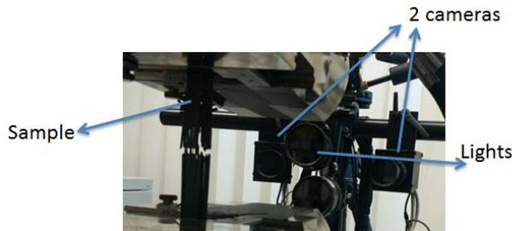
**Figure 8.4. View of the sample and DIC equipment.**
