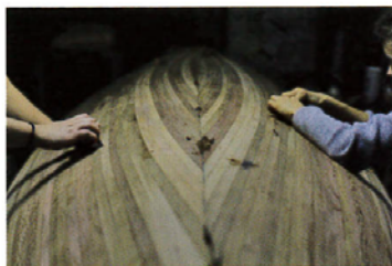
Students recognizing the benefit of a sharp plane as they round out the hull.
