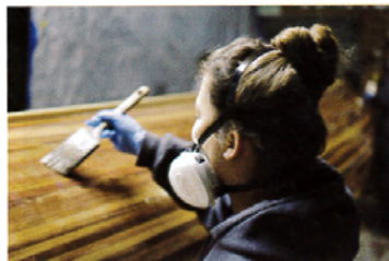
A student applying the finishing touches of epoxy to the outside hull.
