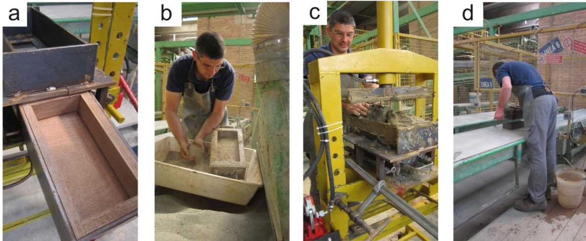
Figure 2: Main stages of soft-mud process for hand-moulding brick production.
