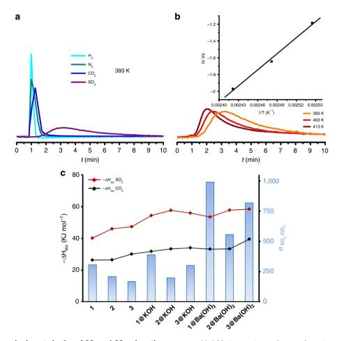
Figure 4 | Thermodynamic characterization of SO<sub>2</sub> and CO<sub>2</sub> adsorption processes. Variable temperature pulse gas chromatography results as:
