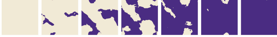
Figure 3.1: Transformation of the topography displayed in Fig. 1.6 a) to a stack of level sets. The height h decreases from left ( h_{min} ) to right ( h_{max} ). White areas represent material, blue represents void areas.
