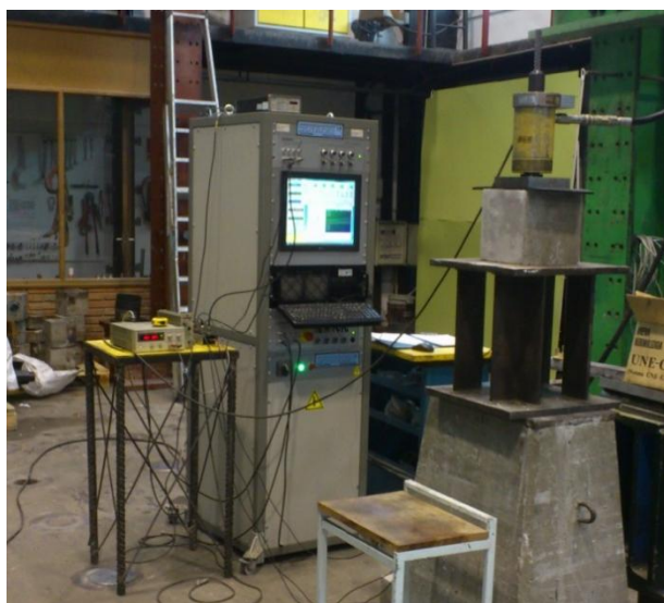
Figure 1. General view of the bond test arrangement
