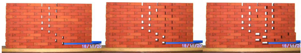
Figure 5. Different collapse mechanisms examples during the same test.
