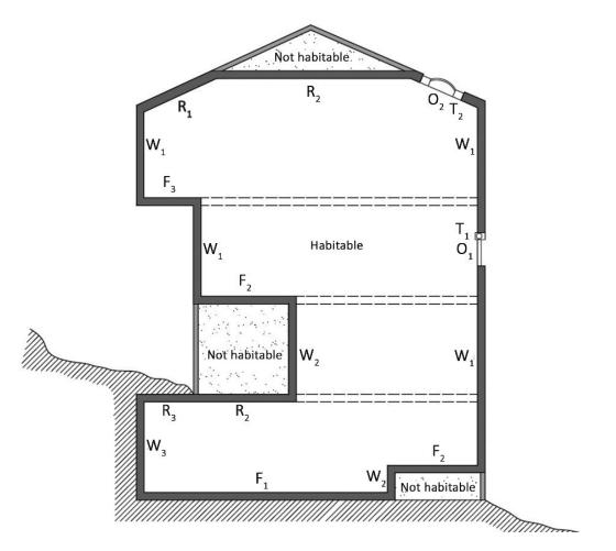
Figure 1: Composition of the thermal envelope of a building: Vertical external walls (W); Horizontal roofs (R); Floors (F); Openings (O); and Thermal bridges (T) [13].
