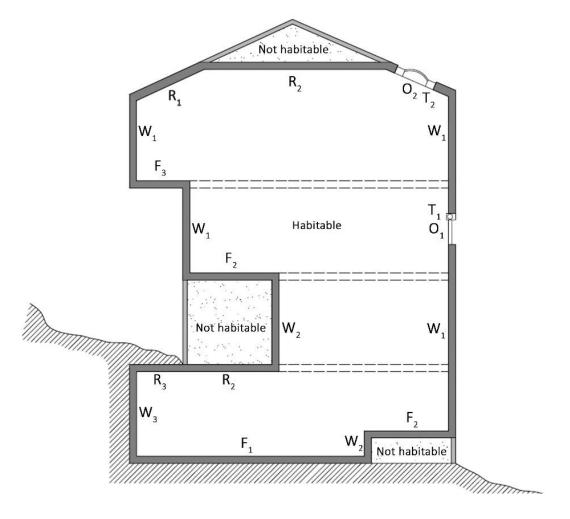
Fig. 16. Composition of the thermal envelope of a building: Vertical external walls (W); Horizontal roofs (R); Floors (F); Openings (O); and Thermal bridges (T) (RD 314/2006).
