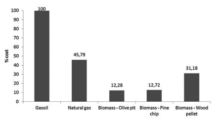
Fig. 7. Costs. Gasoil is the reference fuel.
