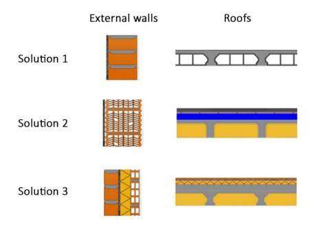
Fig. 17. Elements and materials used. Graphic details.
