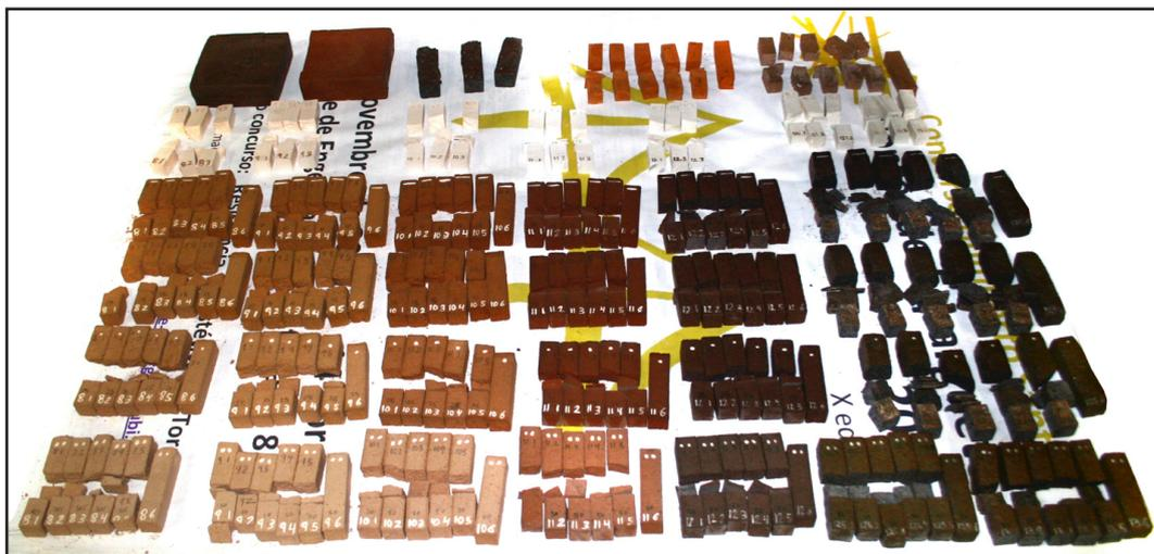
**Figure 7.** Panoramic view of the test samples subjected to 3-point flexural-strength test.
