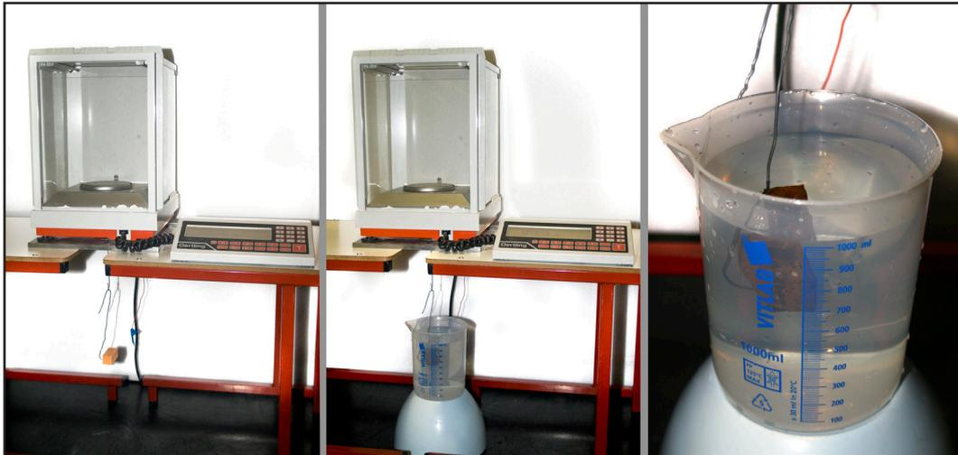
**Figure 14.** Oertling VA204 balance with a capacity of up to 200g and resolution of 0.0001g, with which the samples were weighed dry (left), immersed, and saturated (centre and right, respectively).
