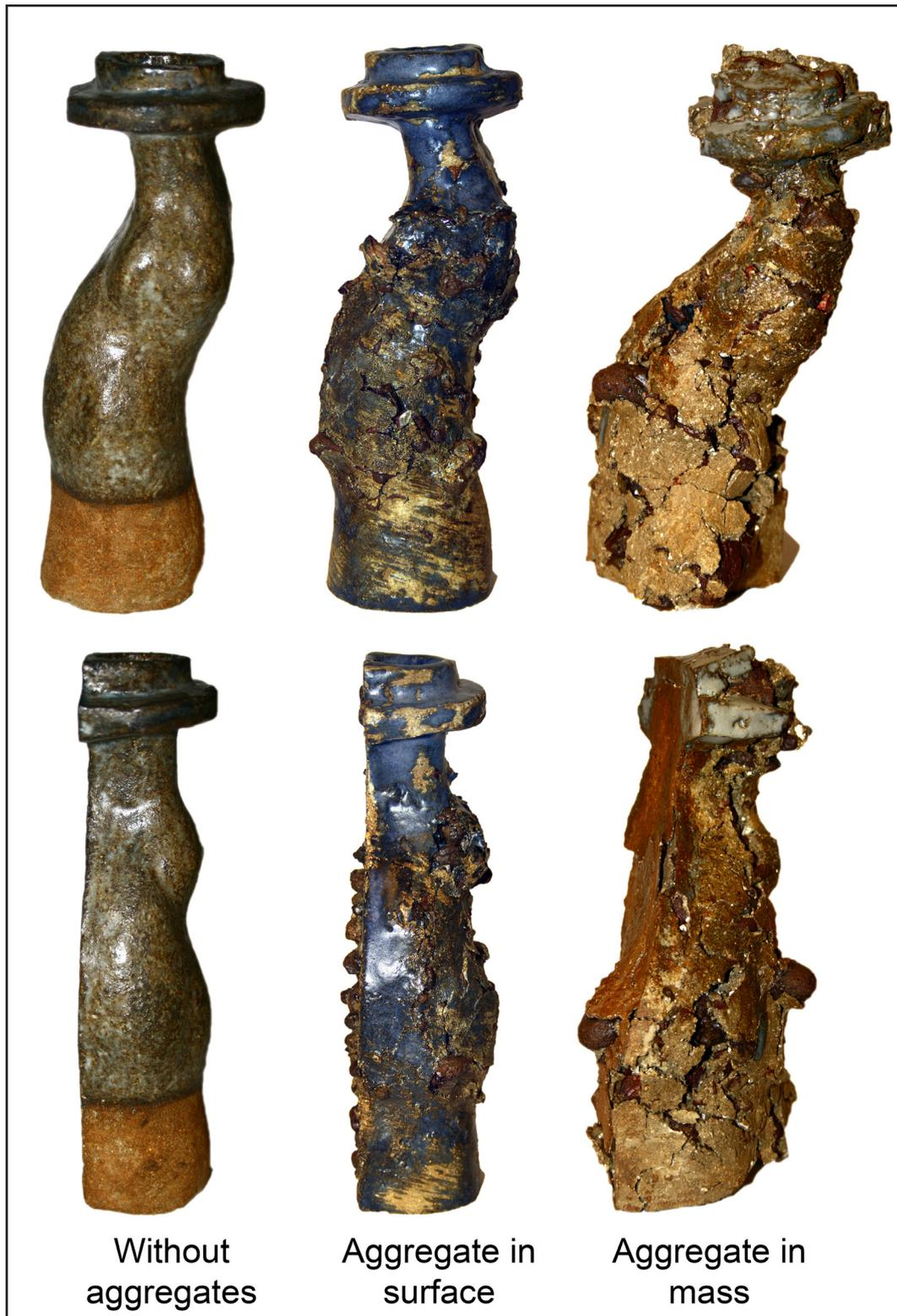
**Figure 30.** Front and side view of three pieces 19.5 cm tall, fired at 1260°C; from left to right: mixed refractory pastes without PAN aggregate, same mix of pasta with the aggregate used in surface encrustations, and same mixture of pastes with the aggregate used in the composition in mass, as a degreaser. Note the volumetric and textural variation according to the use of the aggregate. Pieces by Duran Suárez and Montoya Herrera.
