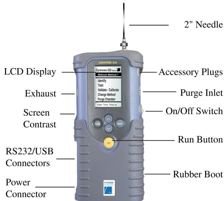
Figure 5. Electronic tongue Cyranose 320 by Cyranose Sciences, California, USA.
