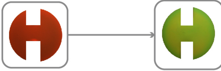
Figure 2. Images showing the change in color of the pSi sample during degradation and the mask used to select pixels for image analysis.
