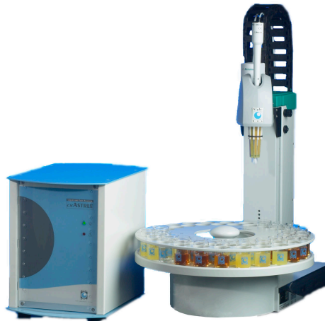
Figure 4. ASTREE electronic tongue from Alpha MOS ( www.alpha-mos.com ).
