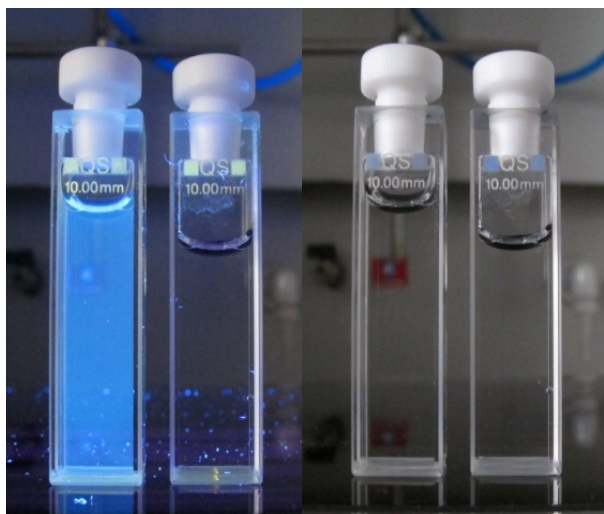
Figure 5. Photographs of Cdots solutions under visible light (right) and UV beam of 365 nm (left) in comparison with only water.
