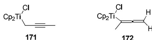
Scheme 131. Simplified titanocene (III) substituted propargyl complexes.
