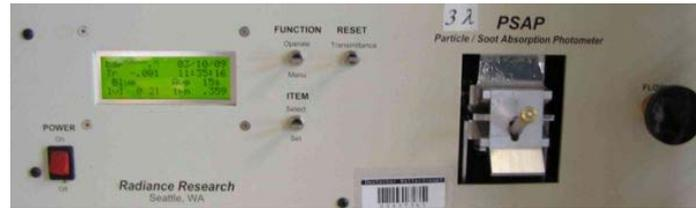
**Figure 3.6:** Particle Soot Absorption Photometer (PSAP).
