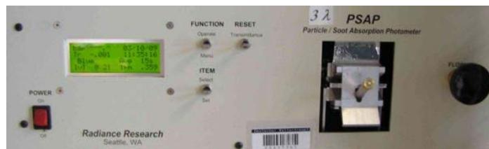
**Figure 3.6:** Particle Soot Absorption Photometer (PSAP).
