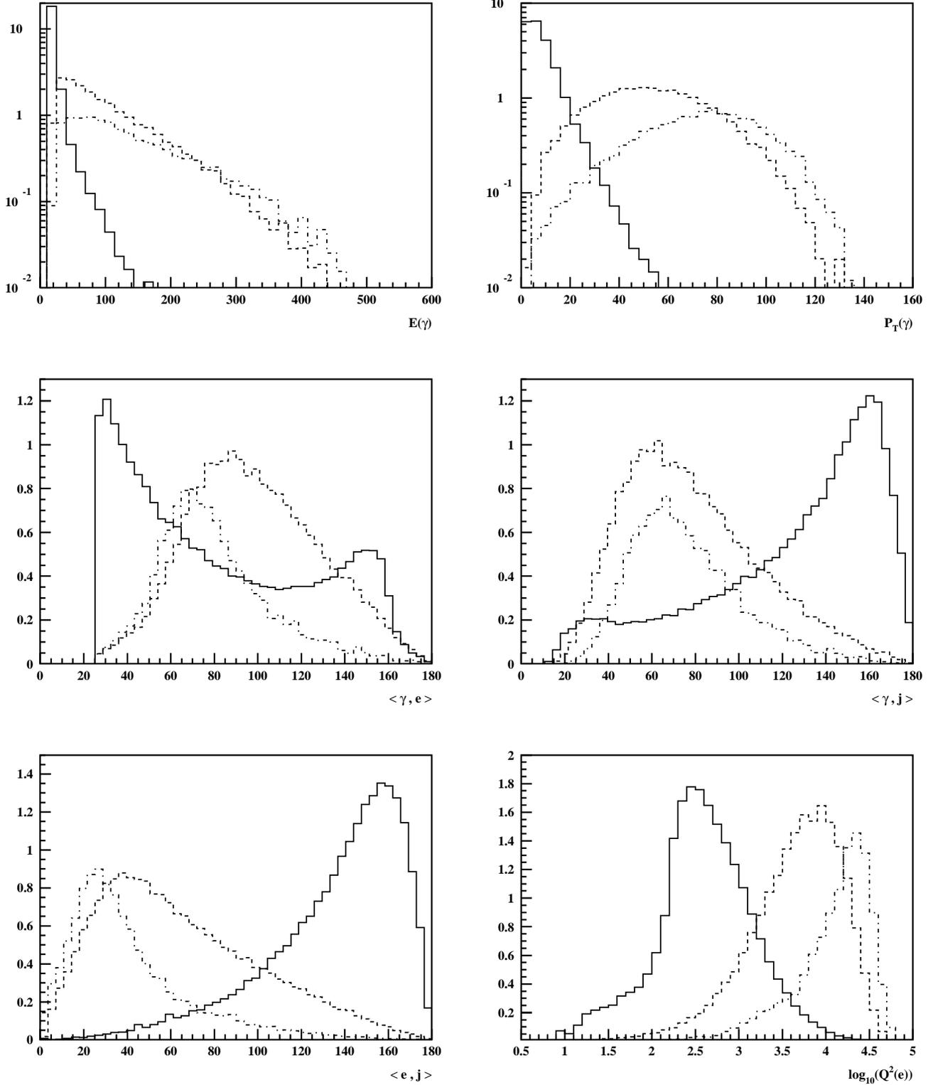
Figure 2: *Differential cross sections (pb) for the process  $ep \rightarrow e\gamma X$  at HERA, with only acceptance and isolation cuts. The solid line is the Standard Model contribution and the dash (dot-dash) line correspond to 10000 times the  $\sigma_1$  ( $\sigma_2$ ) anomalous contributions.*
