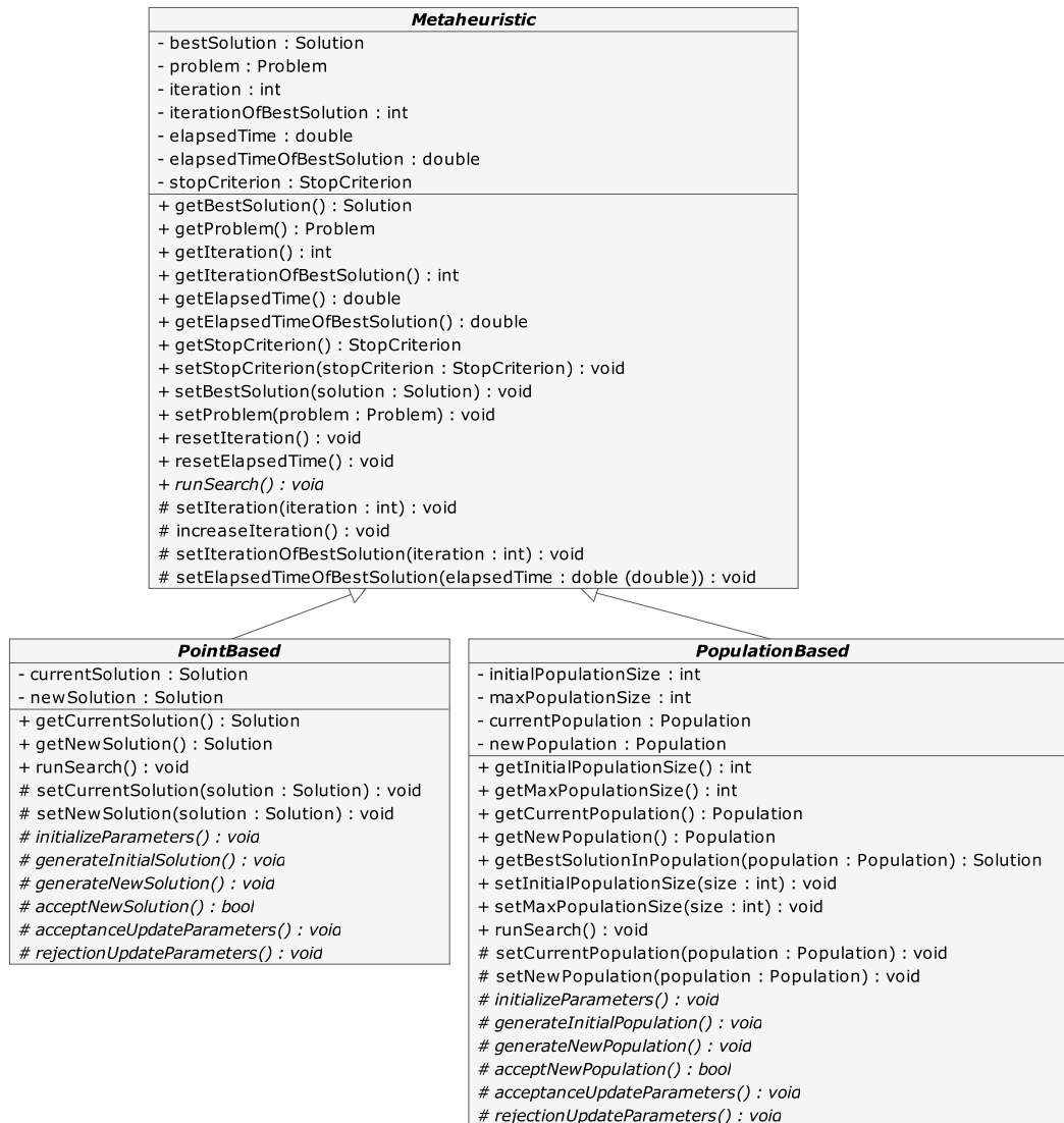
Figure 5.7 – MODO Optimization Package . Main metaheuristic-related classes introduced in [191]. In the MODO Optimization Package, these classes have been replaced by “Algorithm”, a more generic one, but with similar features. Some of the ideas introduced in [191] regarding metaheuristics have been adapted to subclasses of Algorithm, like, e.g., a specific class for population-based algorithms, with methods inspired in the PopulationBased class shown here.
