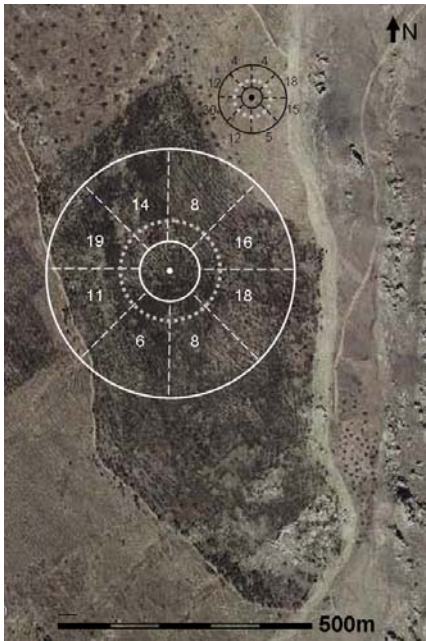
Figure 1: Eddy tower locations as bull's eyes in Non intervention (white) and Salvage Logging (black) treatments. For each tower, according to the Flux-Source Area model of Schmid (1994) during periods of relative static stability (periods where measured fluxes are generated most distantly to the eddy tower) defined in terms of the friction velocity ( 0.2 \text{ m s}^{-1} < u_* < 0.4 \text{ m s}^{-1} ) and sensible heat flux ( H < 0 ), the maximum source location is denoted by the circle of grey dots. Similarly, the white circles denote the near- and far-limits of the 50% source area isopleths. According to Schmid (1997) a flux source point located on or outside the 50% source area boundaries would have to be from 5 to 10 times stronger than the point of maximum source weight,
