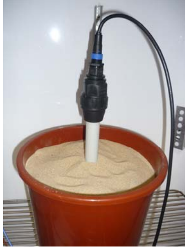
Figure 5. Sensing probe buried in the lysimeter
