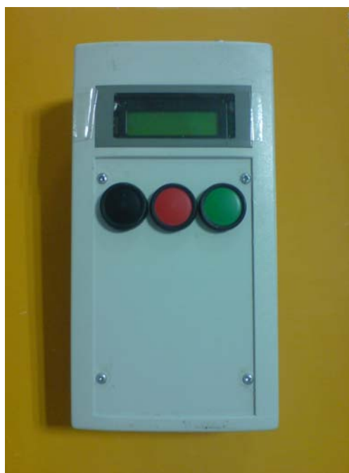
Figure 9. Portable instrumentation for gaseous carbon dioxide determination
