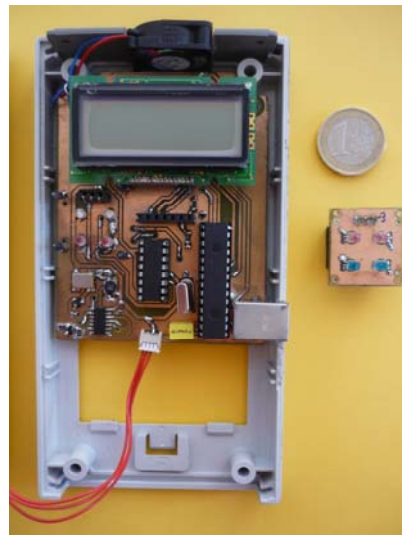
Figure 8. Inside of the portable instrument and photodetectors board.
