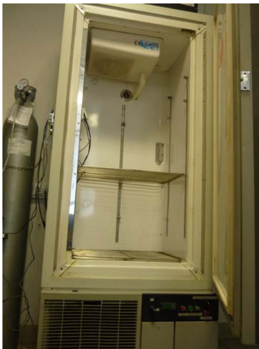
Figure 4. Chamber used for thermal characterization of the instrument
