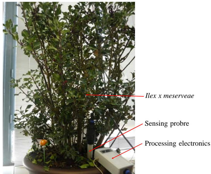
Figure 6. Instrument setup for near-root oxygen measurement.
