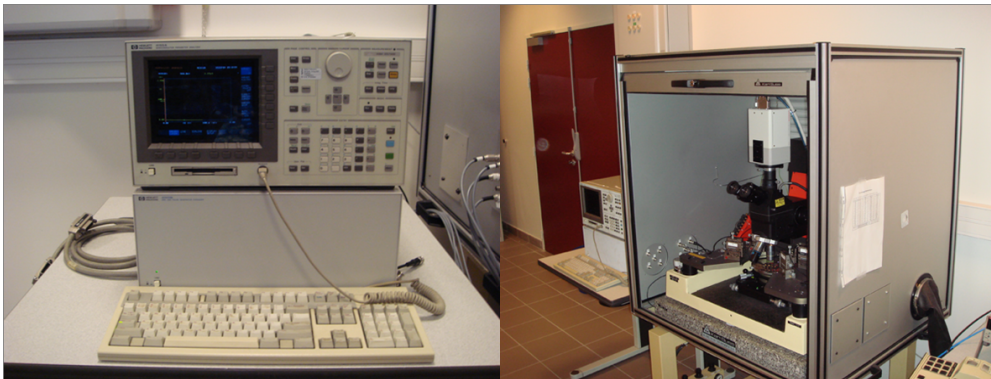
Figure 7.16: HP4155A Semiconductor parameter analyzer (left hand side). Karl Suss four probe station (right hand side).
