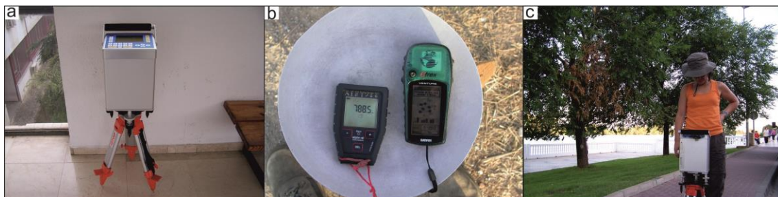
Figure 4.2: Equipment used to acquire gravity data. (a) Scintrex CG-5 Autograv gravimeter on a tripod. (b) Barometric altimeter and Garmin e-trex GPS. (c) Gravity measurement over a field station.
