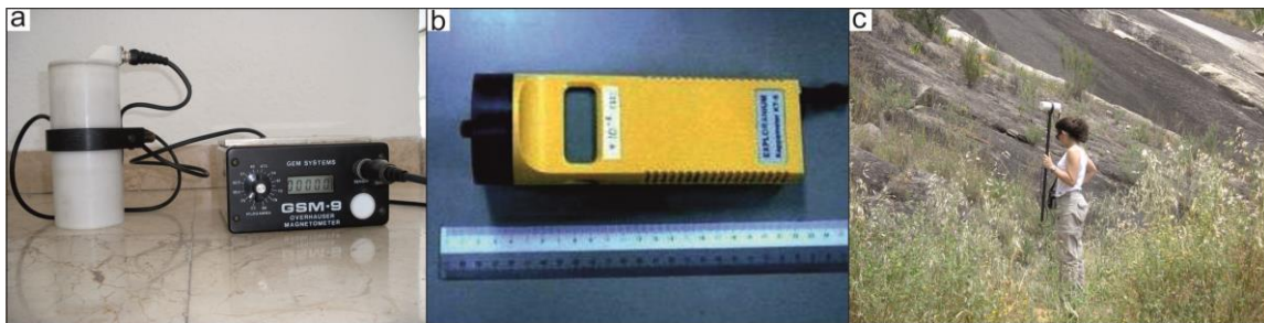
Figure 4.3: Magnetic equipment. (a) Standard GSM 8 proton precession magnetometer. (b) Exploranium kappameter KT-9 Susceptometer. (c) Magnetic data acquisition over a field station.
