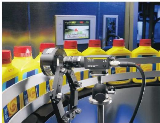
**Figure 5.1.** Inspection system to detect imperfections of the products on the conveyor belt. (Courtesy of *Cognex Corp.*).
