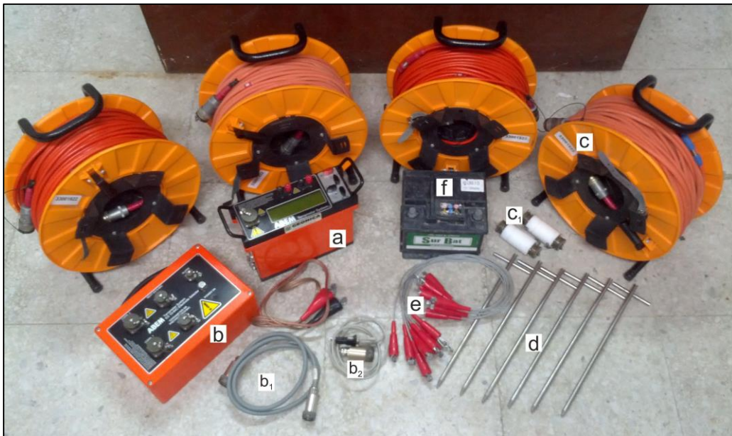
Figure 3.9: Electrical resistivity tomography equipment: (a) Terrameter SAS 4000, (b) electrode selector ES10-64C and (b 1 y b 2 ) cable connectors, (c) cable and (c 1 ) connectors between cables, (d) steel electrodes, (e) connectors cable-electrode and (f) battery supply.
