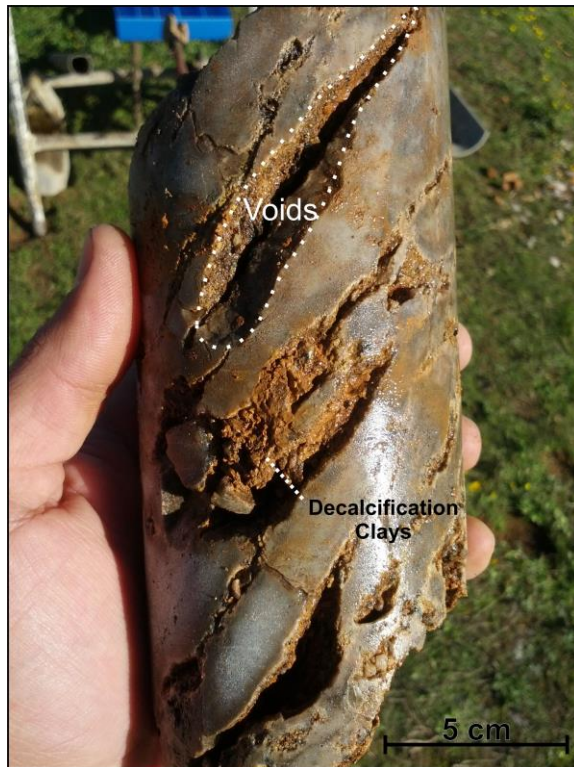
Figure 8.5: Quartzite sample with calcite veins dissolved and decalcification clays filling the voids
