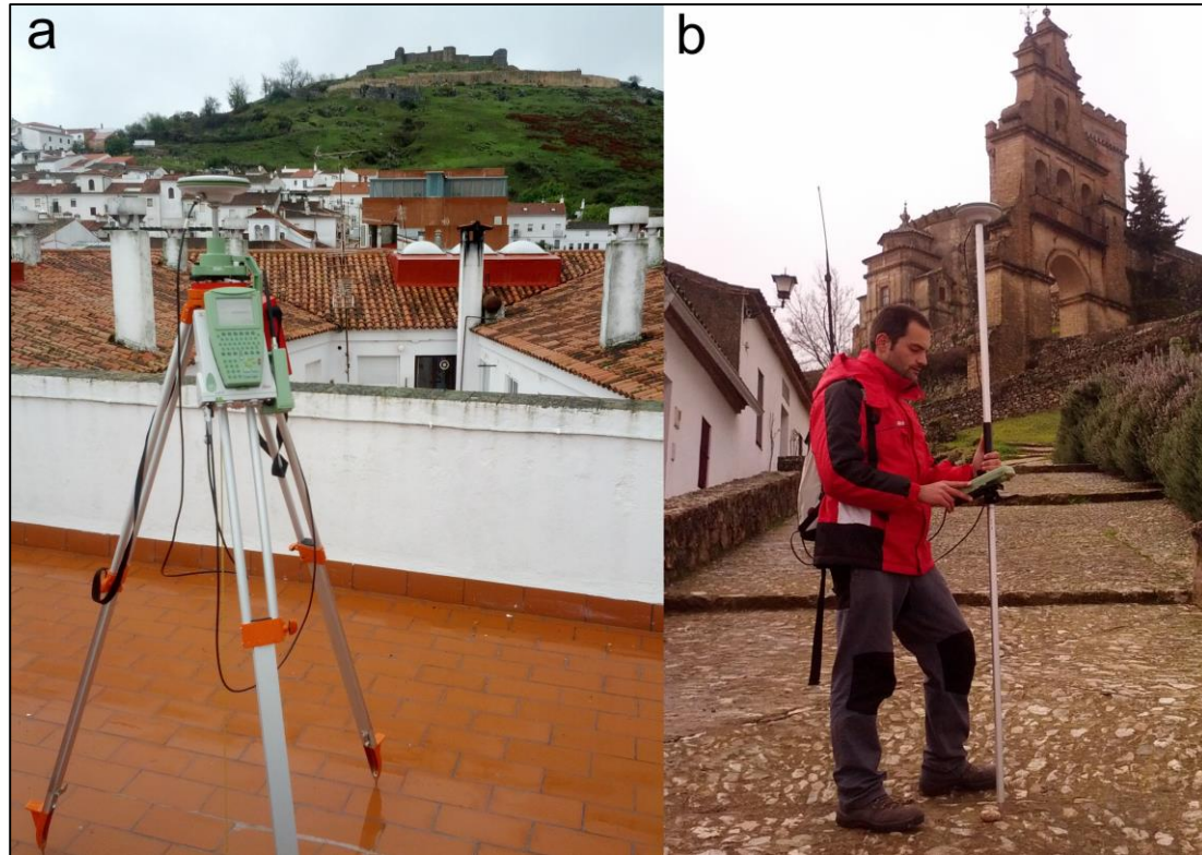
Figure 3.3: Differential GPS Leica 1200 and 1200+ equipment, respectively. (a) Reference Station fixed on a point that covers the whole study area. (b) Taking data into a measuring station with the rover GPS.
