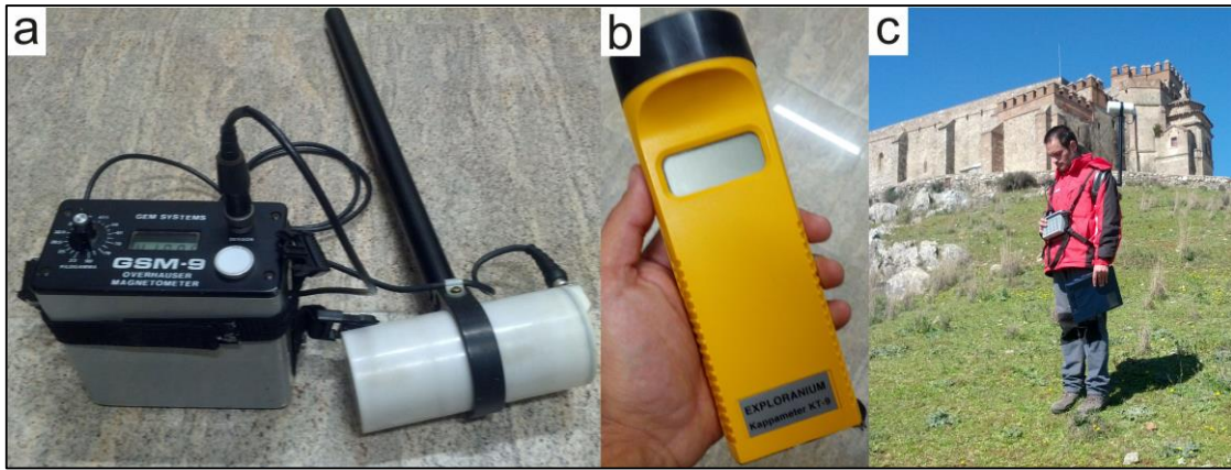
Figure 3.6: Magnetic equipments. (a) GSM - 9 standard proton precession magnetometer. (b) Susceptometer Exploranium kappameter KT-9. (c) Acquisition of a magnetic measure in the field.
