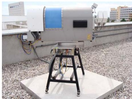
**Figure 3-9: Microwave radiometer.**
