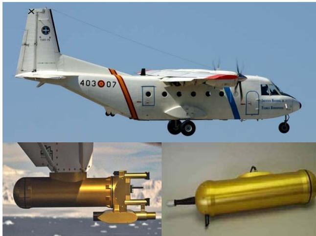
**Figure 8-1: Picture of the INTA CASA C-210-200 aircraft for atmospheric research (from [www.eufar.org](http://www.eufar.org)) and the CAPS (left bottom) and PCASP-100X (right bottom), taken from [www.dropletmeasurement.com](http://www.dropletmeasurement.com).**
