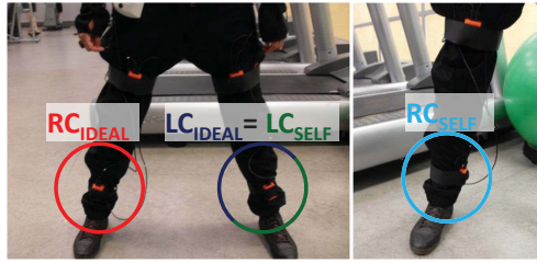
(a) Sensor displacement originated during a user self-placement of the sensors
