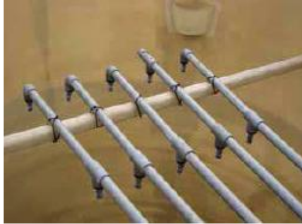
Figure 3.7. Spraying system used in the UF experimental plant.
