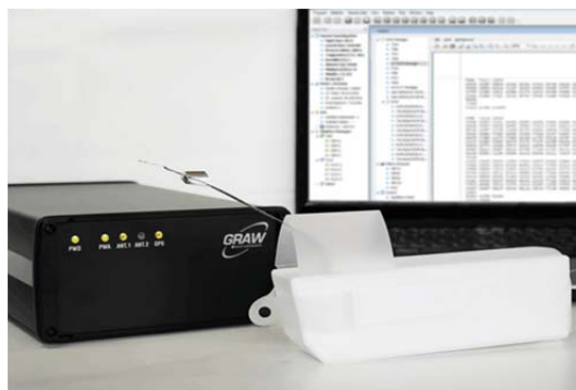
Figure 3.3. GRAWMET software with radiosonde and ground station.
