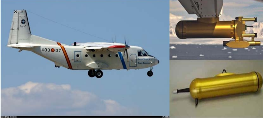
Figure 5.17. Picture of the INTA CASA C-210-200 aircraft for atmospheric research (from www.eufar.org ) and the CAPS (right top) and PCASP-100X (right bottom), taken from www.dropletmeasurement.com .
