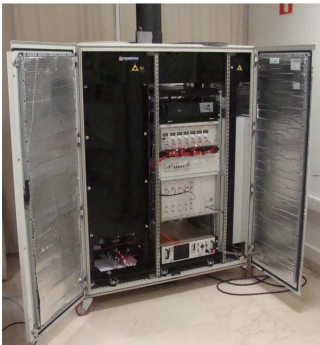
Figure 3.1. Raman lidar system operated at Granada station.
