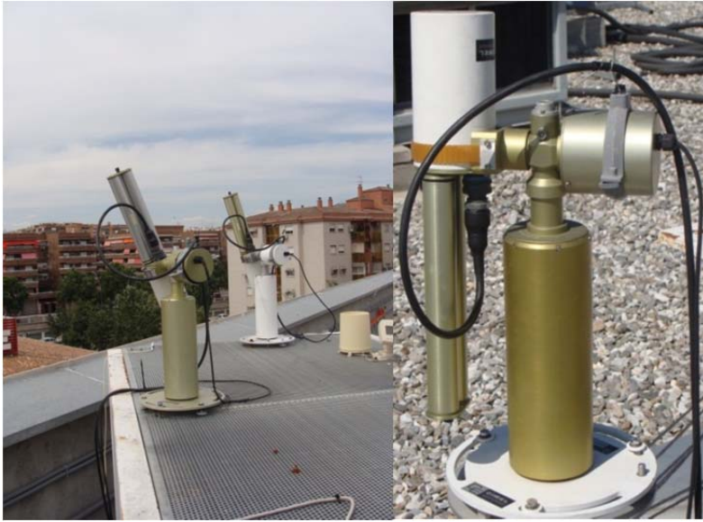
Figure 3.2. Cimel CE 318-4 located at Granada experimental site.
