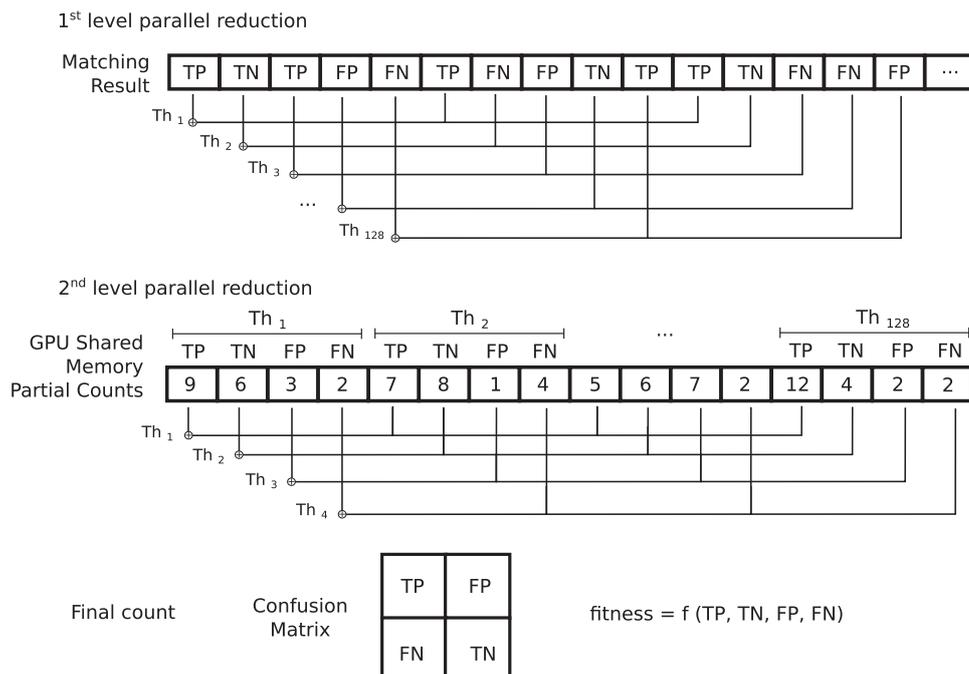
**Fig. 4.** 2-level parallel reduction with sequential addressing.
