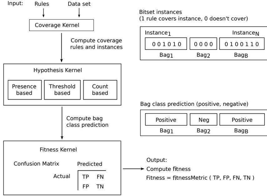
**Fig. 2** GPU evaluation model using three kernels
