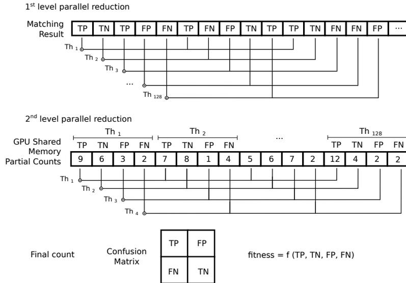
**Fig. 6** Fitness computation using 2-level parallel reduction
