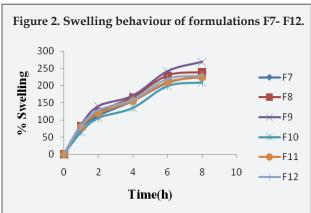
therefore release of all formulations is mainly by Non-Fickian release. It indicates a coupling of the diffusion and erosion mechanism so called anomalous diffusion and may indicate that the drug release is controlled by more than one process. The best fit model for prepared formulation follows Korsmeyer's-Peppas model (r<sup>2</sup>= 0.9942) and n value was found to be 0.183 which signified that release pattern of optimized batch F10 follows the Non Fickian diffusion as shown in tables 3 and 4.
