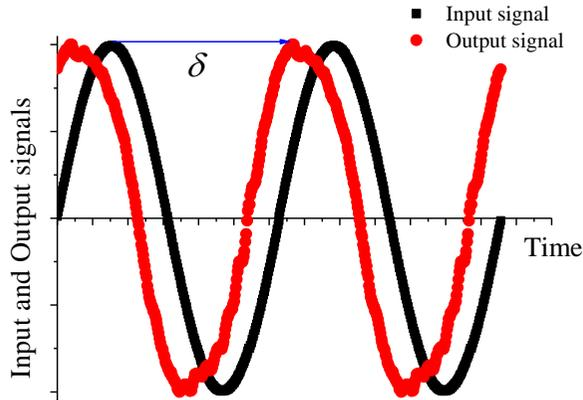
**Figure 4. Output signal as response to an input deformation signal in a small-amplitude oscillatory experiment.**
