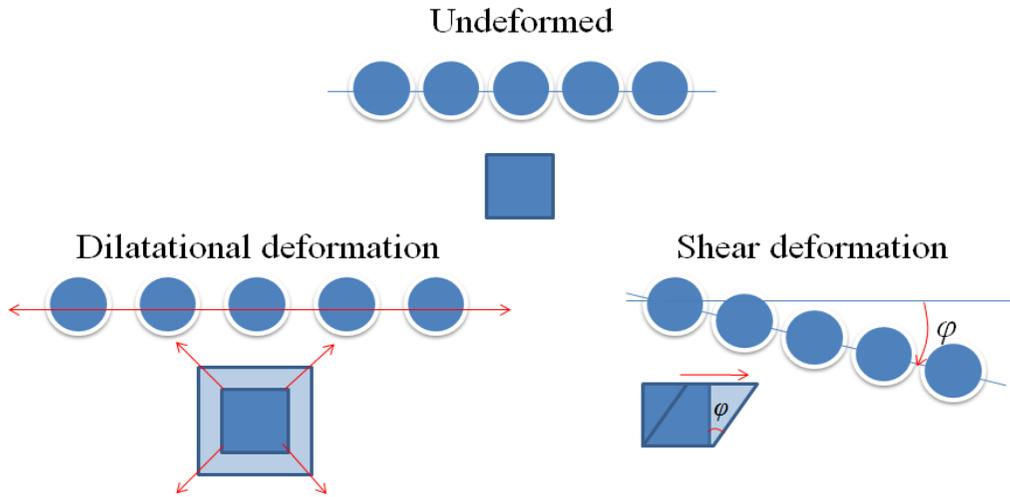
**Figure 3. Schematic representation of both interfacial deformations.**
