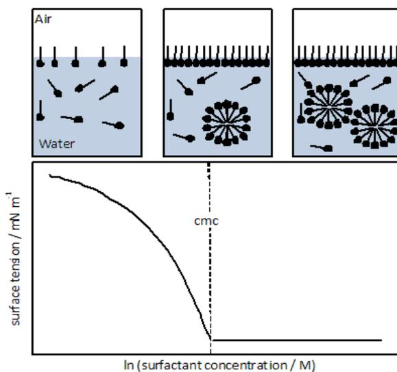
**Figure 2. Structural regions in the equilibrium adsorption process of conventional surfactants: determination of the CMC.**
