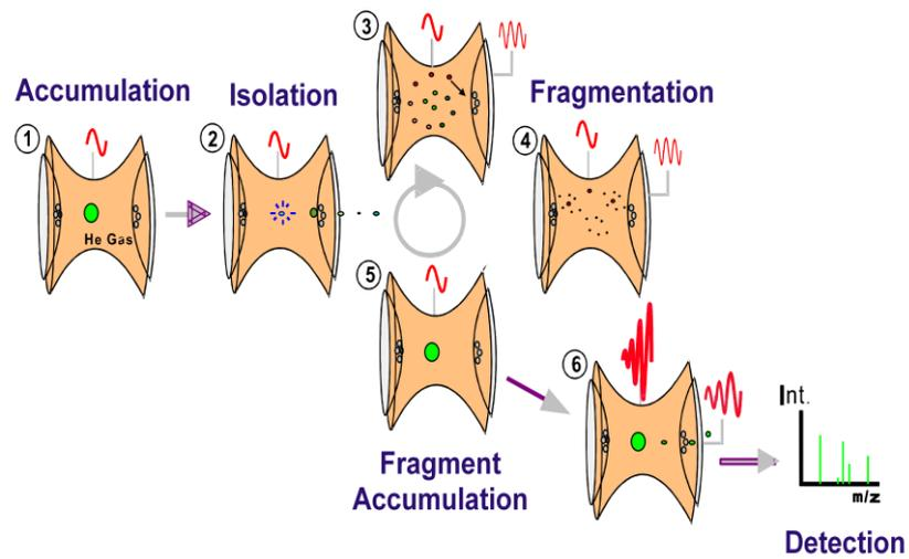
Figure 25. Schematic representation of the IT process
