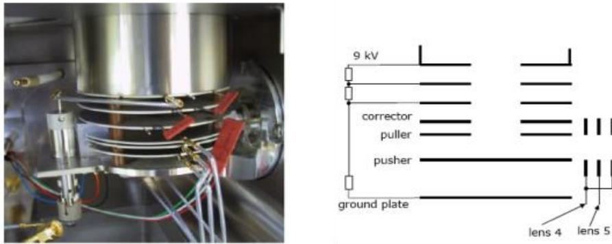
**Figure 22. The zone of orthogonal acceleration of a MicroTOF with a schematic representation of its components**
