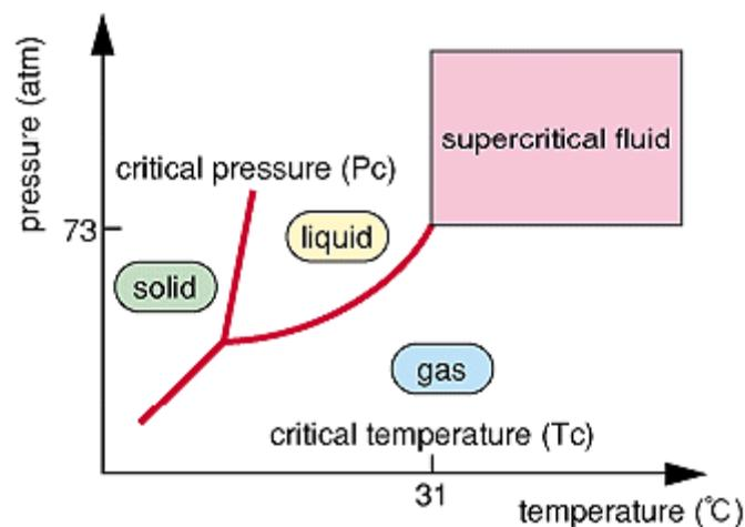
**Figure 13.** Phase diagram of supercritical CO<sub>2</sub>
