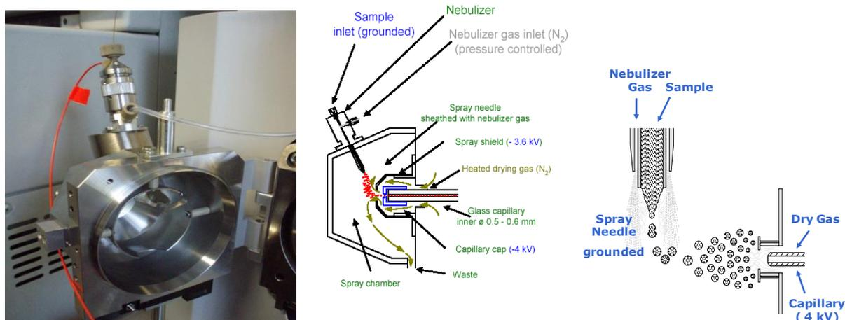
**Figure 19. ESI ion source with its schematic diagram**
