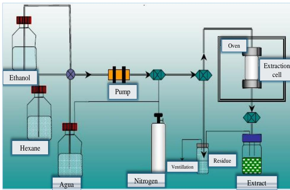
**Figure 12.** Schematic diagram of the PLE system
