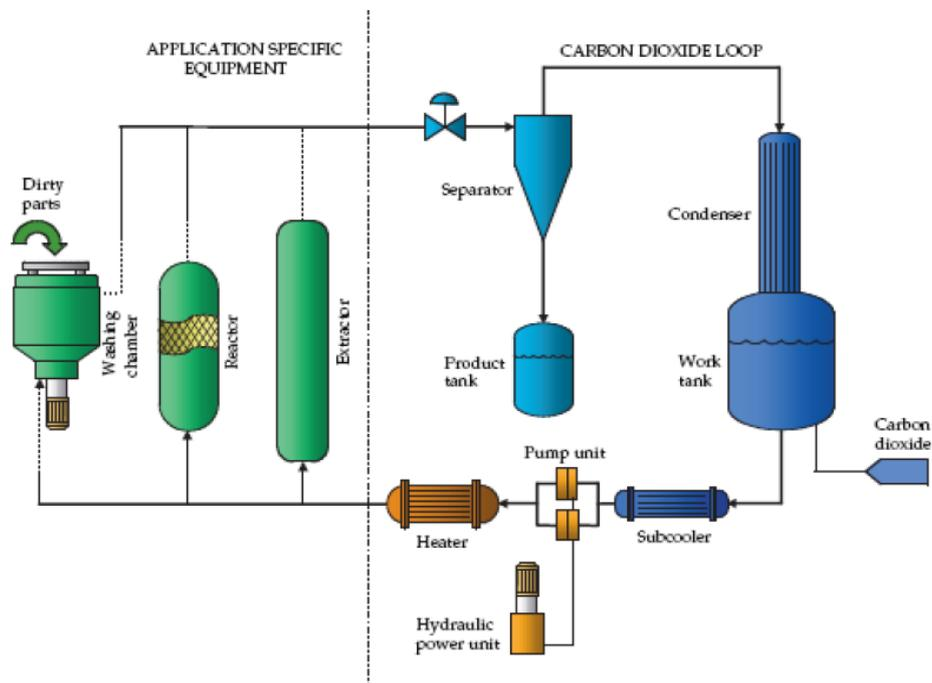
**Figure 14.** Schematic diagram of PLE system
