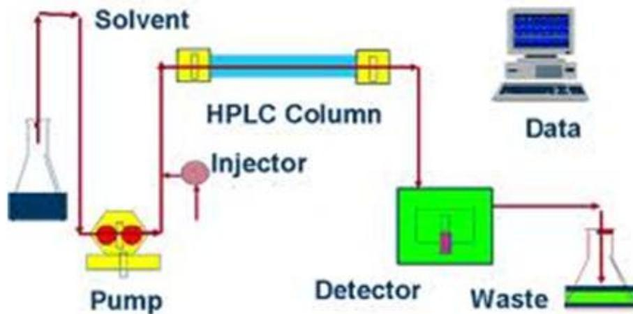
**Figure 16.** Schematic diagram of HPLC system
