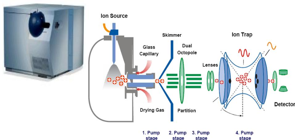
**Figure 24. IT Mass analyser with its schematic diagram**
