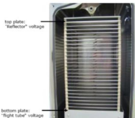
**Figure 23. Image of the last part of the flight tube showing the reflector**
