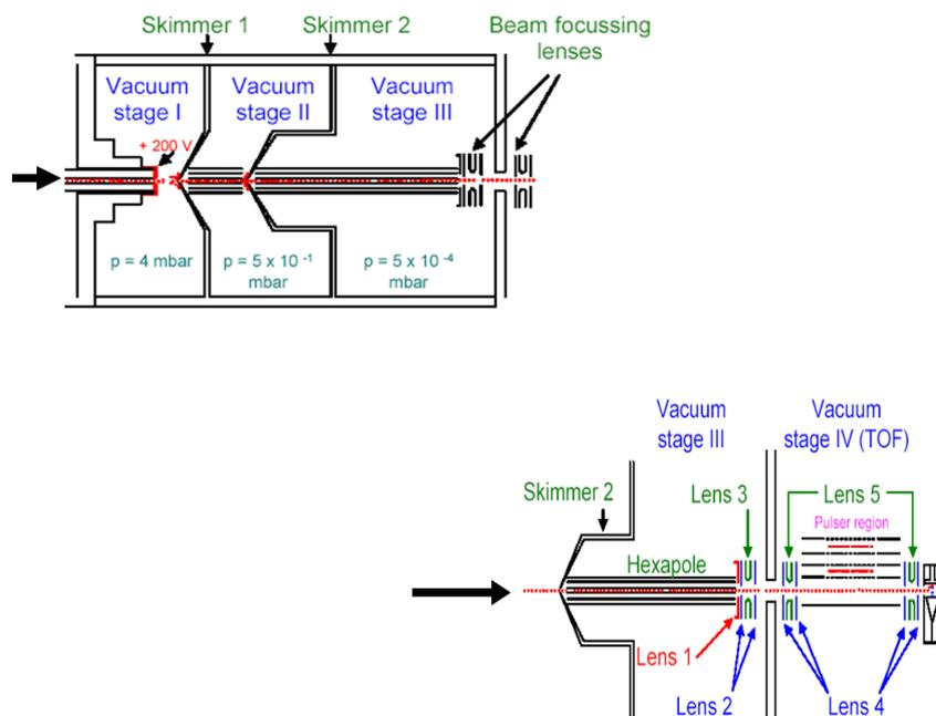
**Figure 21. Schematic diagram of the transfer optic unit**
