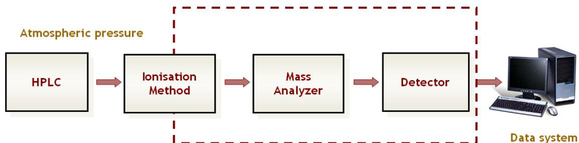
**Figure 17.** Combination of separative technique with mass spectrometry
