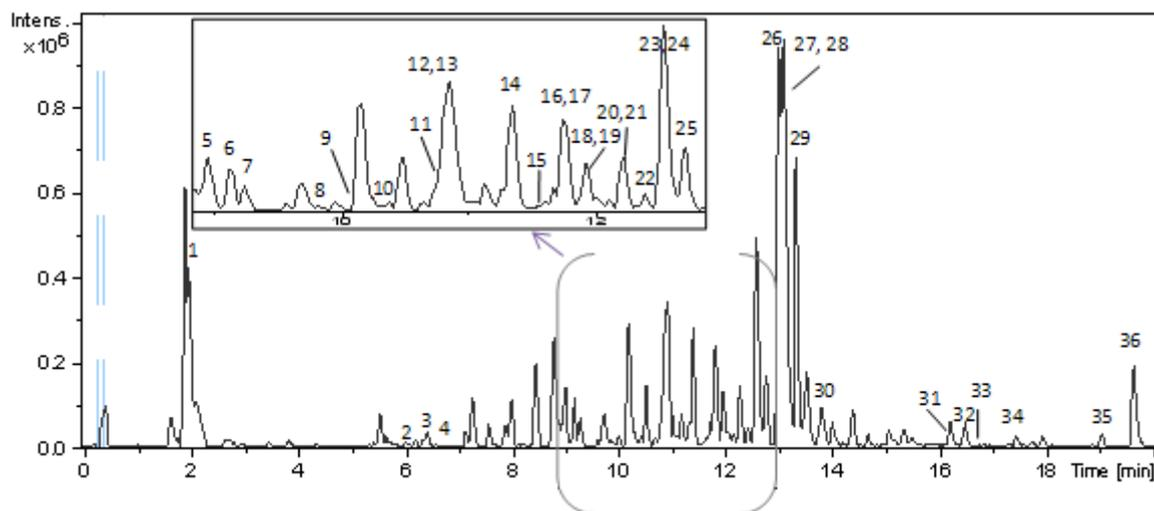
**Figure 3. BPC of an olive leaf extract obtained under the optimized condition of MAE.**
