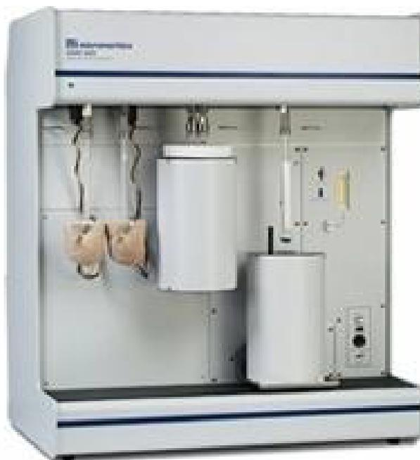
**Figura 29.** Analizador Micromeritics, ASAP 2020 Physisorption (Micromeritics® Instrument Corporation, Norcross, GA, USA)
