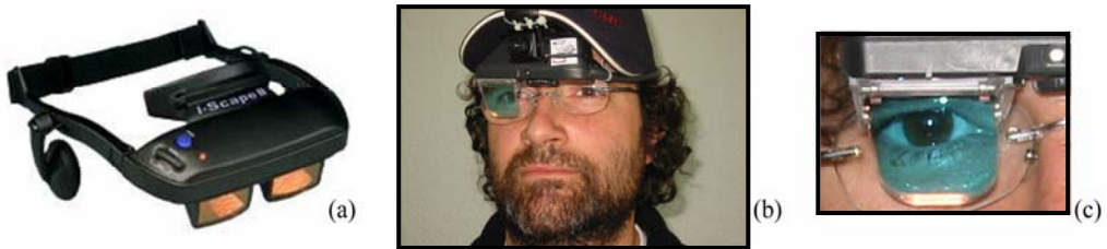
Figura 2.3.- (a) Virtual IO glasses; (b) NOMAD ND2000; (c) Detalle del visor del NOMAD ND2000.
